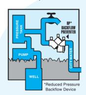
supply connection to the well system. For a list of approved assemblies, contact your local water supplier (listed on the back of this brochure).
