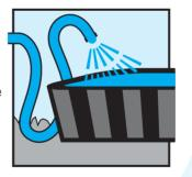
Heating, Cooling, and Fire Sprinkler Systems: Heating, cooling and fire sprinkler systems that use water from the potable supply pose a hazard because water within those systems often sits stagnant for long periods of time or may have chemical additives.
