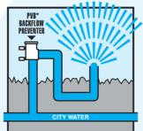
\*Pressure Vacuum Breaker (can also use Double Check Valve Assembly)
