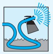
other non-potable substance creates a cross connection that can allow the contents of the container to backflow into the water supply.
